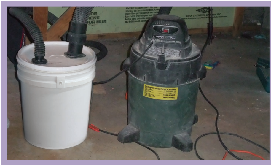
Picture 1 – Vacuum cleaner installation to reduce dust emission in the house
